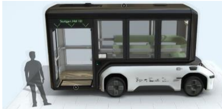
Figure 22 - Intermodal passenger Pod with road Pod carrier (Fig.: DLR)
