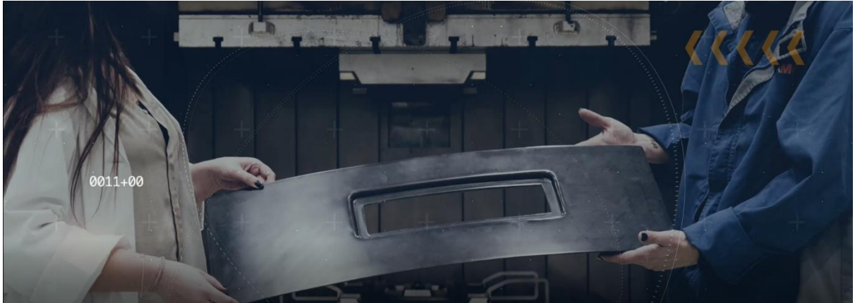
Figure 2 - View a 1/3 scale composite part for a door leaf
