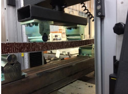
Figure 1 - Bending test of insulated pillars
