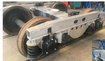
Complete bogie with aluminium frame –mock up
