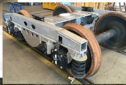
Aluminium bogie 3D model, assembly and prototype.
