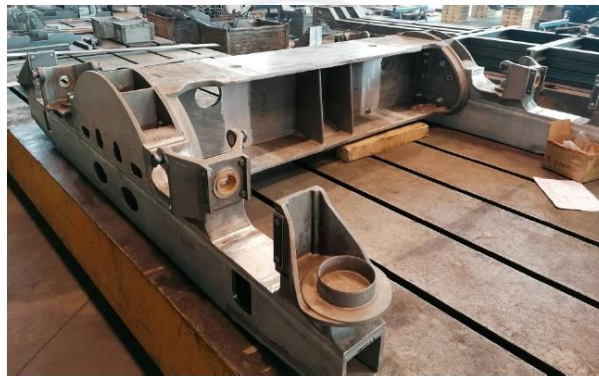
Complete bogie with aluminium frame –mock up
