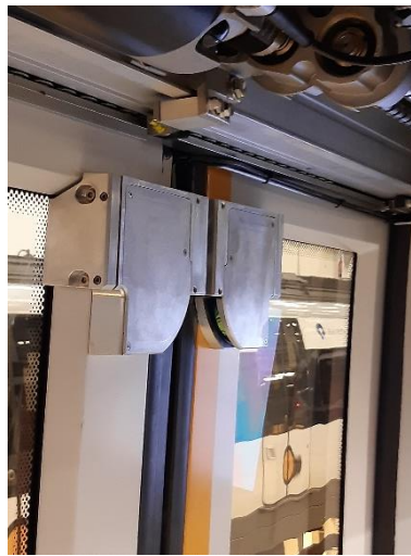
Figure 3 - View of laser scanner for touchless obstacle detection
