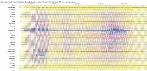
Operational visualizations (decision support results) Space-time diagram with platform/train occupancy
