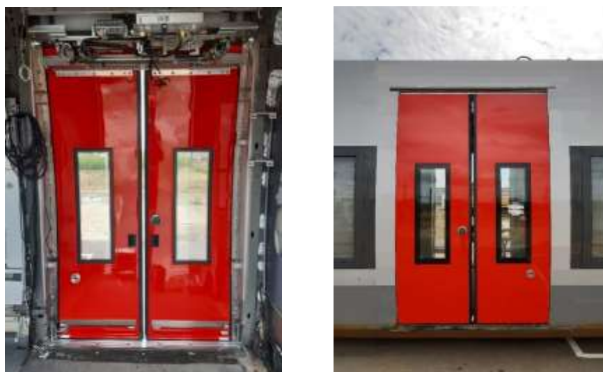
Door mounted on a static SNCF train equipped with door leaves, swinging arm and handles developed with PIVOT2
