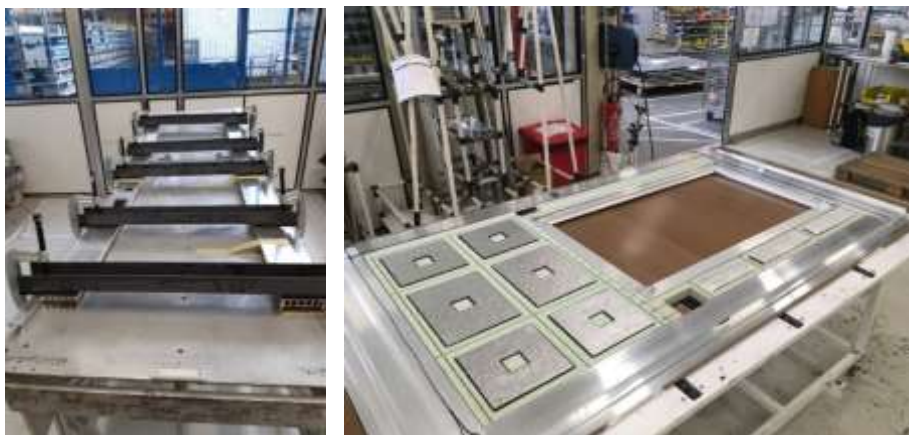
Bonding of the insulated pillars (left). Innovative filling material (right).
