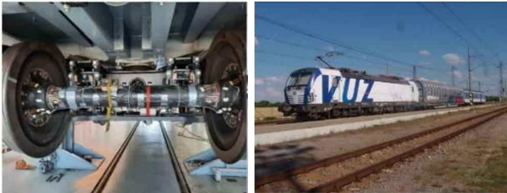
Setting of the measuring wheel for the track tests (left). Train set during the test on the VZO (right).
