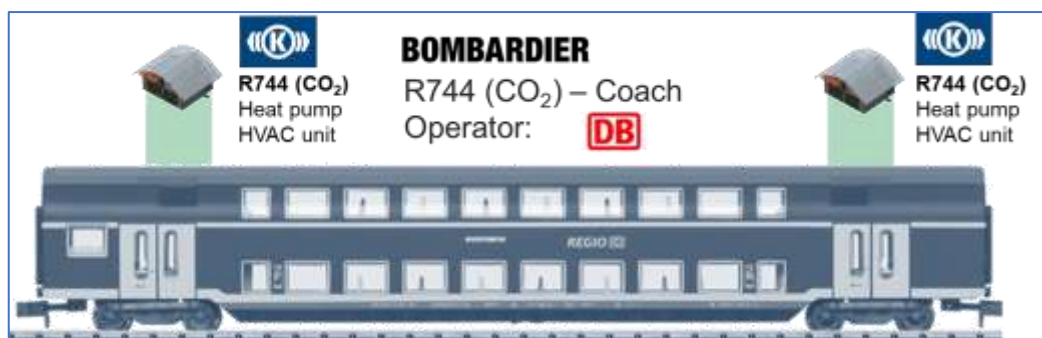
HVAC units mounted on a double-deck regional train
