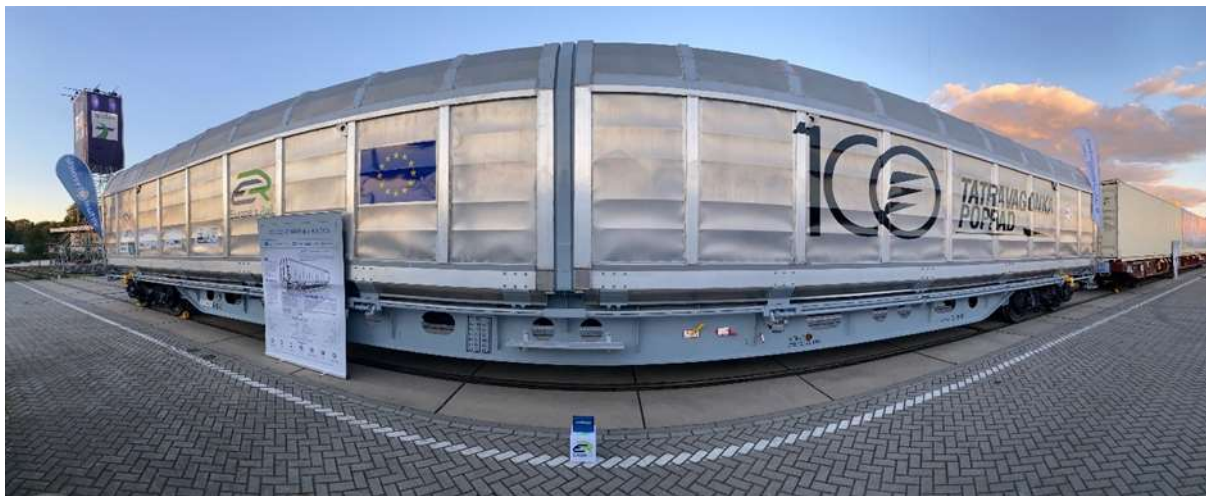
Core Market Wagon at InnoTrans 2022 including T&E Equipment, ProDisc Axle, SiSet Silet Wheelset, and an Automatic Coupler
