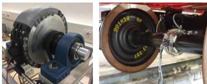
Axle Mounted Power harvester in the laboratory test-bench and installed in a wheelset for field tests in Minden
