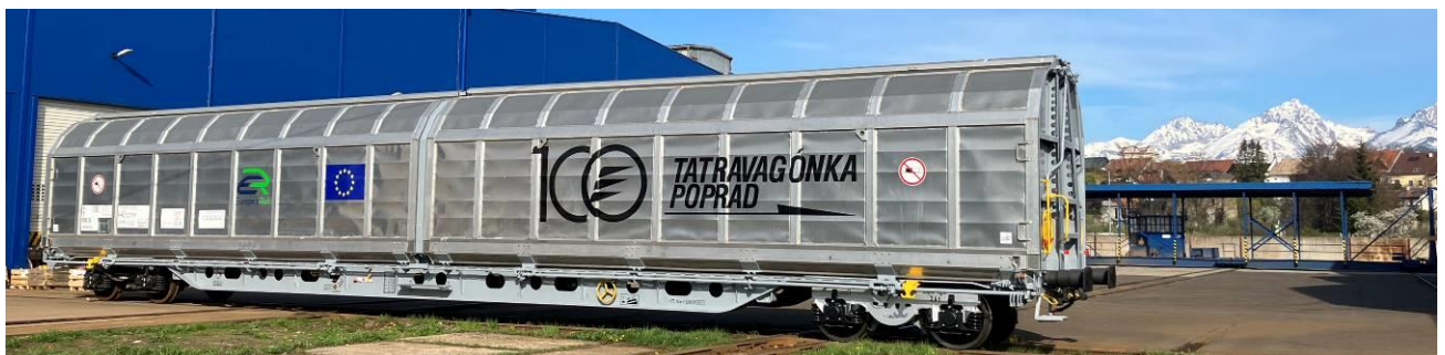
CMW with FR8RAIL bogie with aluminium bogie frame
